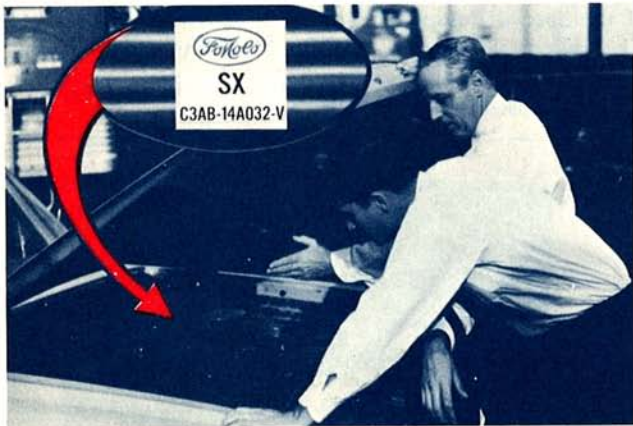
Figure 5—Identifying Wiring Looms
