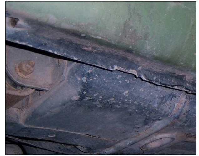
In this example paint was applied at a slightly different angle and distance which produced a wider black paint application and less runs on the floor pan close by.
