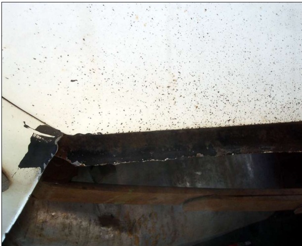
Rear quarter panel pinch weld black out applied after rear valance was pulled into the body at the bottom edge.
