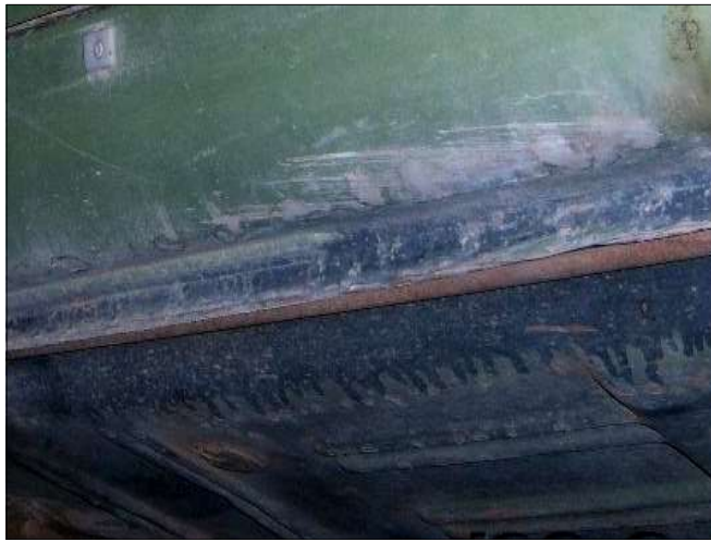
Closely applied example of pinch weld blackout on this example produced runs of black paint on floor near gun and less overspray inward on the floor
