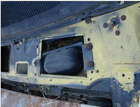
Cowl under cowl cover was body color or blacked out with engine compartment black depending on the car's build date. Black paint is worn on example
