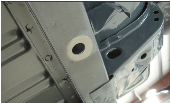
On this restored example it shows the round dolly make with soft edges and the much fainter design left from the pinch weld black out that produces more of a U shaped pattern since it was only applied from one direction.
