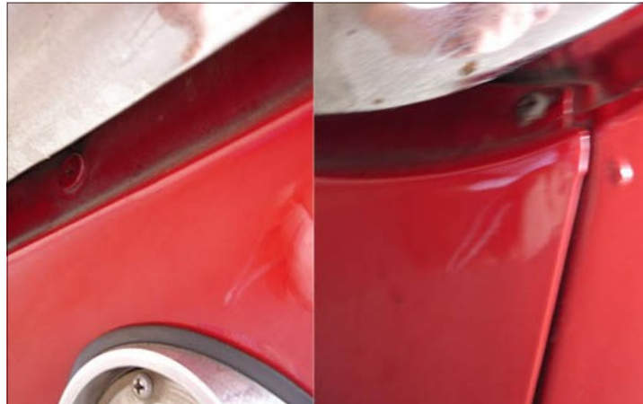
Example of the painted and unpainted screws holding the rear valance to the taillight panel on a later car.
