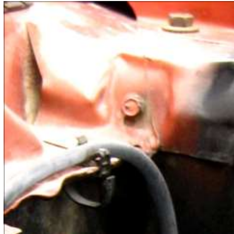
Typical location of black paint to cowl body color. Soft line/edge = not taped. Picture, above right, shows the post mid March painted splash shield screw.
