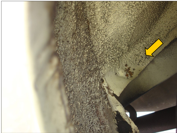
Example of amount of direct exterior color on the visible surface over sound deadener. In right picture
