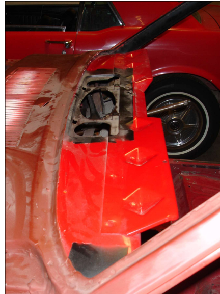
Dash paint details. Top coat red exterior over black interior paint
