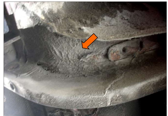
Heavy application on frame and floor section.
