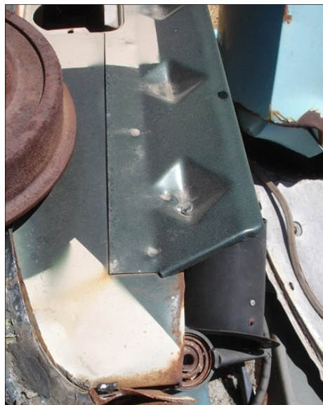
Dash paint details. Top coat green exterior over tan interior paint
