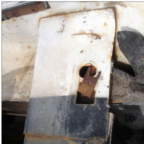
Typical location of black paint to cowl body color. Soft line/edge = not taped. Picture, above right, shows the post mid March painted splash shield screw.
