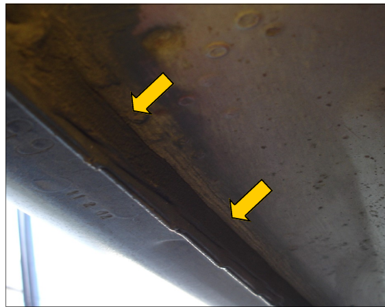
Rocker panel to floor seam chalking
