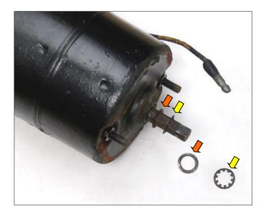
The picture above shows a motor with the retainer and washer slid down the shaft and another retainer and washer for size reference.
