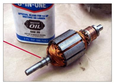
If the contact for the brushes on the rotor are scored too badly, do not use. Clean the rotor shafts with a cloth. If there is too much corrosion on the long end, use some 400 grit sand paper to remove. This is the end that the fan goes on so try the fan for easy fit. Put a drop of SAE 20 oil on each end of the shaft. Use oil designed for electric motors. Make sure the thrust washer, red line, is installed on the long end of the shaft.
