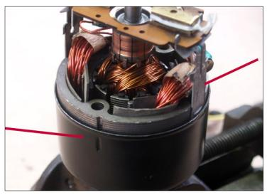
Install the stator into the fan shaft end aligning the stator with the alignment marks and an indent. Do not force it in – yet. Yes, you can get it in 180 degrees out so use the wire lead end of the housing to make sure the marks are correct. The wire lead end with the leads placed in the access hole will only fit one way.
