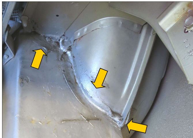
Green-Chalking applied but not spread or wiped
