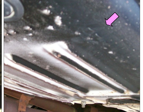
This car received a heavy (more overspray) coat close to the pinch weld likely due to paint gun angle
