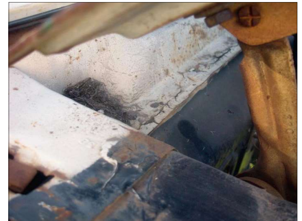
Typical location of black paint to cowl body color Soft line—not taped
