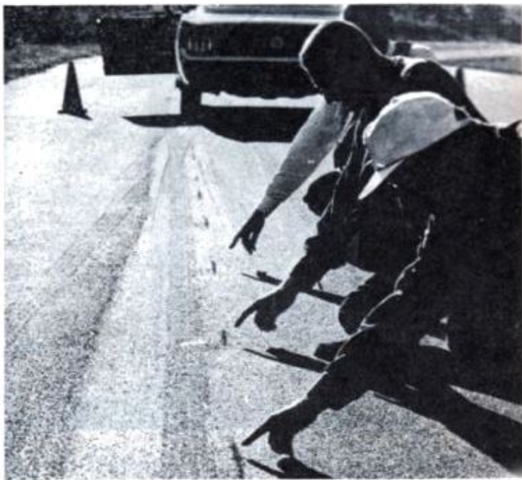
THE BRAKING WHEEL HOP after Mustang's handling runs left this series of short skid marks on track surface. These punishing stops were hard to control
