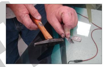
With a quick strike of a small tack hammer the bracket popped off. Looking back it would have been a good idea to wrap the outer (non-striking surfaces) of the hammer head with duct tape or a couple of coats of masking tapes to reduce the chance that I would scratch the glass as I slid it across the surface of the glass to strike the razor.
