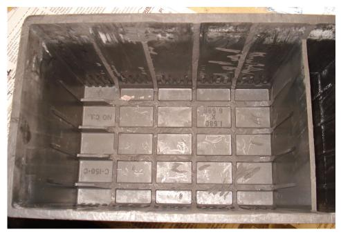
I mentioned that you do not need to remove the fill cap nipples to remove the lid, but you may need to trim them down for battery clearance. I went ahead and cut the nipples off flush with the cut I had made to remove the lid. In these pictures, there are still two nipples that need to be trimmed. The cutoff wheel works great for this.
