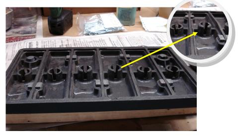
Here is the other tedious step in this process. You need to drill and tap a hole in the underside of the lead posts for a threaded stud. The word of caution here is that the lead is tricky to drill because the swarf tends to fill the flutes on the drill and can abruptly bind the drill bit in the hole. Don't even think about drilling a small pilot hole
