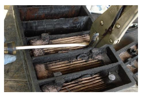
I placed the plates in a plastic bag for disposal. My local battery distributor will accept these plates and the bottle of acid at no charge and I assume they recycle the plates and safely dispose of the acid.
