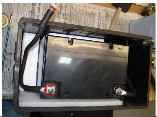
Note that I trimmed the remaining case partition with the cutoff wheel to make it level with the case of the new battery. This is necessary so that there is clearance to route the cable. I also used some scrap styrofoam to fill the gaps between the new battery and the case so that it wouldn't slide around or rattle. I didn't bother with padding the top as I didn't want to interfere with the fit of the lid and I thought the chances of the new battery hopping up
