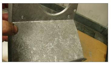
Depending on the finished surface you produced, you can now choose to finish the part by applying a single coat of a satin clear or leave it as it is. This additional layer of paint can lock all the levels together and provide a slightly smoother
