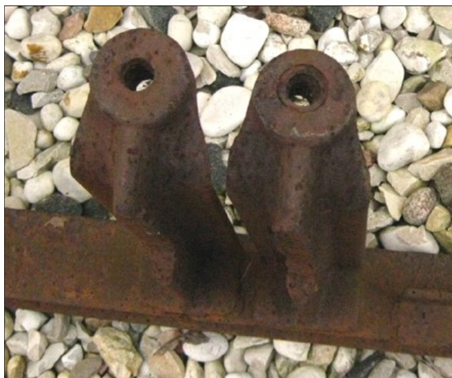
Here is a close up of the rear mounting stands (in this example from 69-70—see last page for explanation) . At this point (and one further forward) the car was bolted to the dolly.
