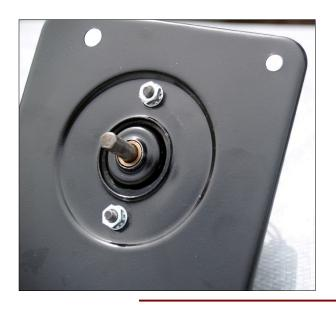
Install the mounting plate on the two long screws over the seal. Note the offset left hole and the plate edges turned away (towards the engine compartment). Not shown is the wiring grommet and leads located on the top when the motor is installed properly. The factory motors used two each of the following hardware items to retain the plate to the motor:
