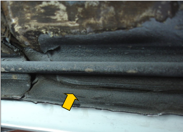
Rocker panel to floor sealant. This is one of the heavier and messier examples of the application.
