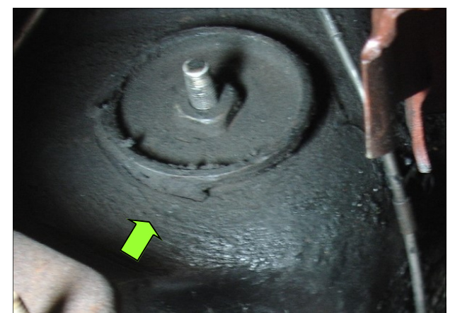
Rear seat belt anchor example. Applied around the anchor then wiped around the anchor
