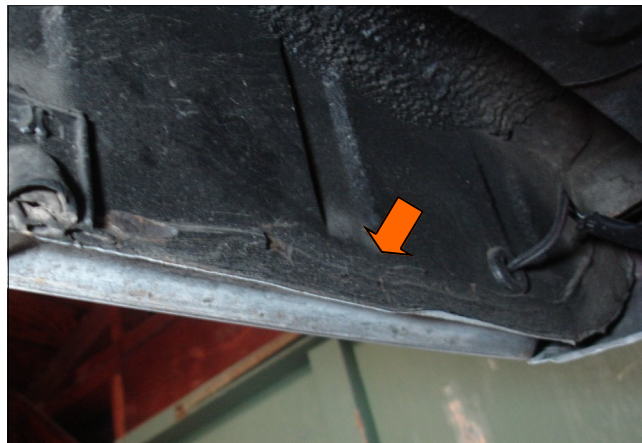
Trunk drop sealant applied and wiped at the bottom edge of the trunk drop to quarter panel pinch seam.
